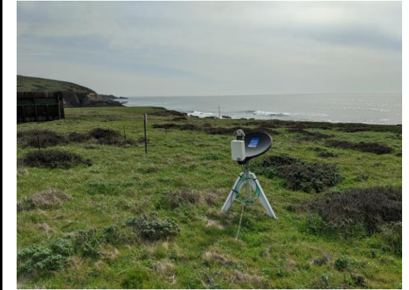
CW3E MRR (K-band) 3km range, 100m resolution
