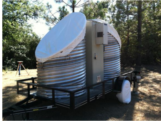
NOAA FMCW (S-band) 10km range, 40m resolution
